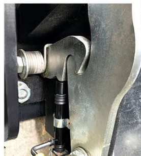
Automatic lock in up-right position
